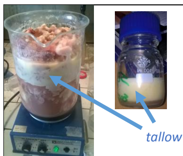
Figure 3. Rendering process of waste beef tallow.
